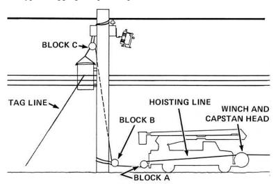
ii. If the bucket can reach the pole and transformer position, the transformer may be installed to the winch line using this approved sling method:
