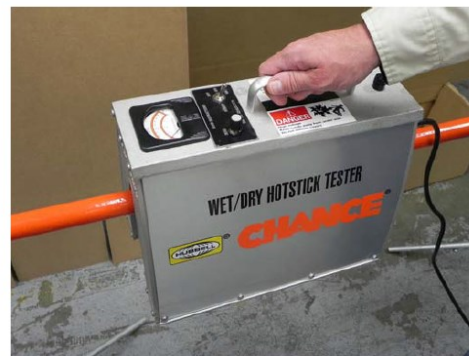
To pass the OSHA wet test, water must bead up rather than wet out the surface. Wax or silicone will enhance this property if the surface is in satisfactory condition.
